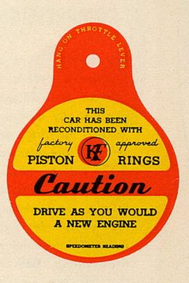
be operated in the manner of a NEW engine. This tag should be attached to the car in a conspicuous place so that the owner will be sure to see it. By providing this warning, you may save yourself the necessity of reservicing the job. Do not let a new piston ring job leave your shop without this tag.
