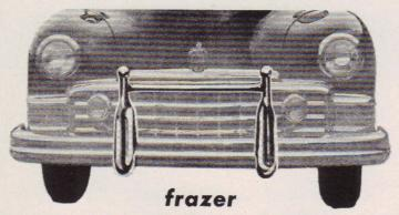
These Radiator Grille Guards consist of two sturdy chrome uprights and a tubular cross bar. These units are installed on the bumper over the standard bumper guards and the linkage connecting the upright guards to the frame help to absorb shock and give excellent protection to the radiator grilles.
