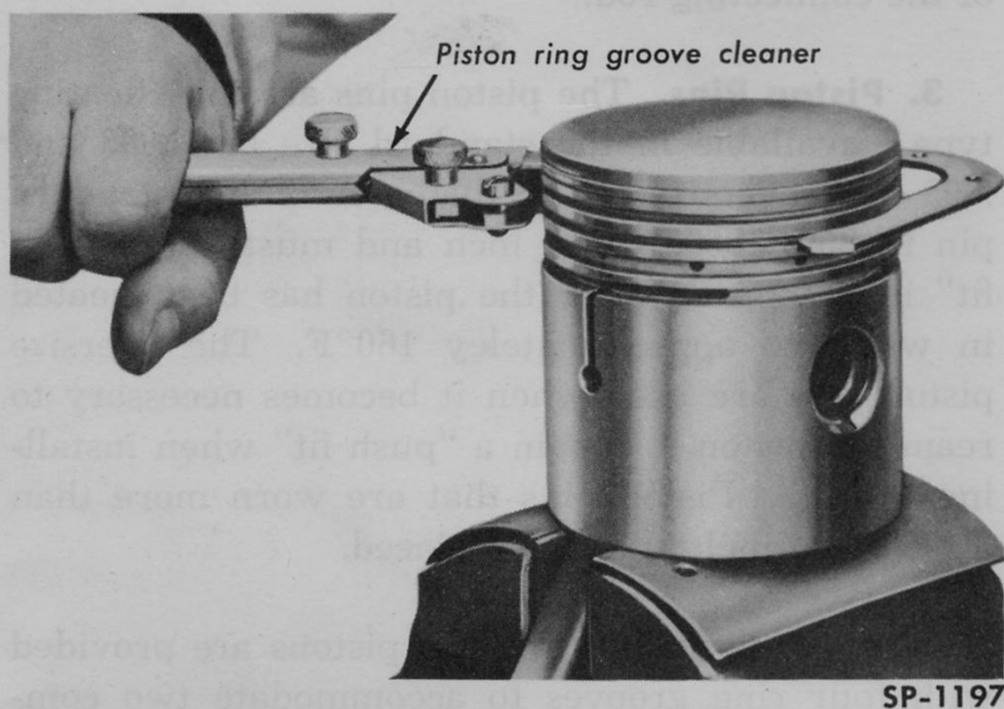
Fig. 42—Cleaning Piston Ring Grooves
