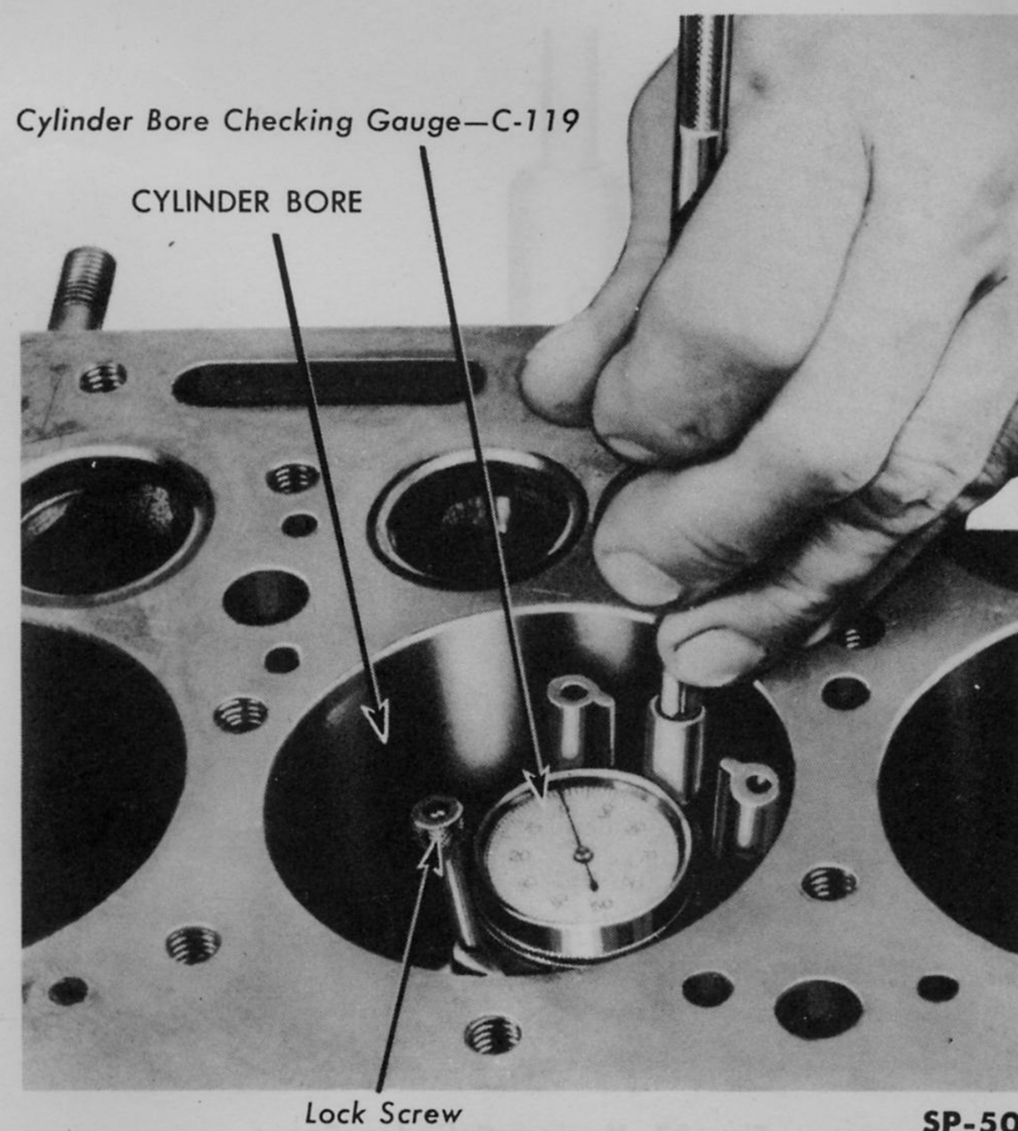
Fig. 36—Checking Cylinder Bore for Taper and Out-of-Round
