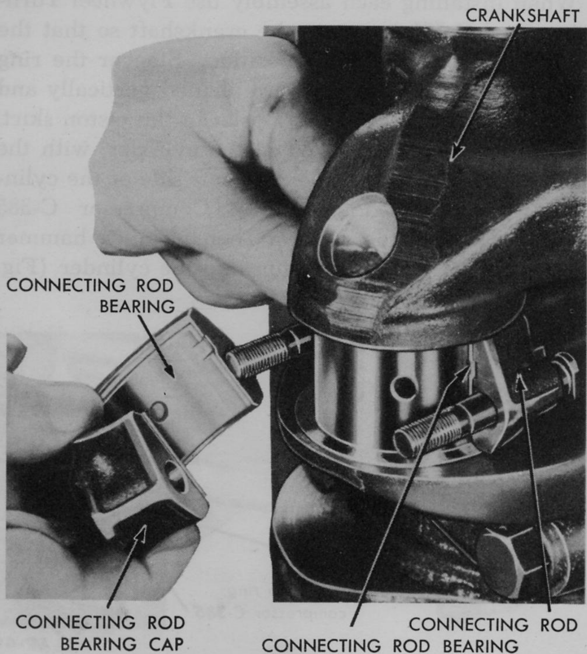
Fig. 95—Installing Connecting Rod Bearing Cap
