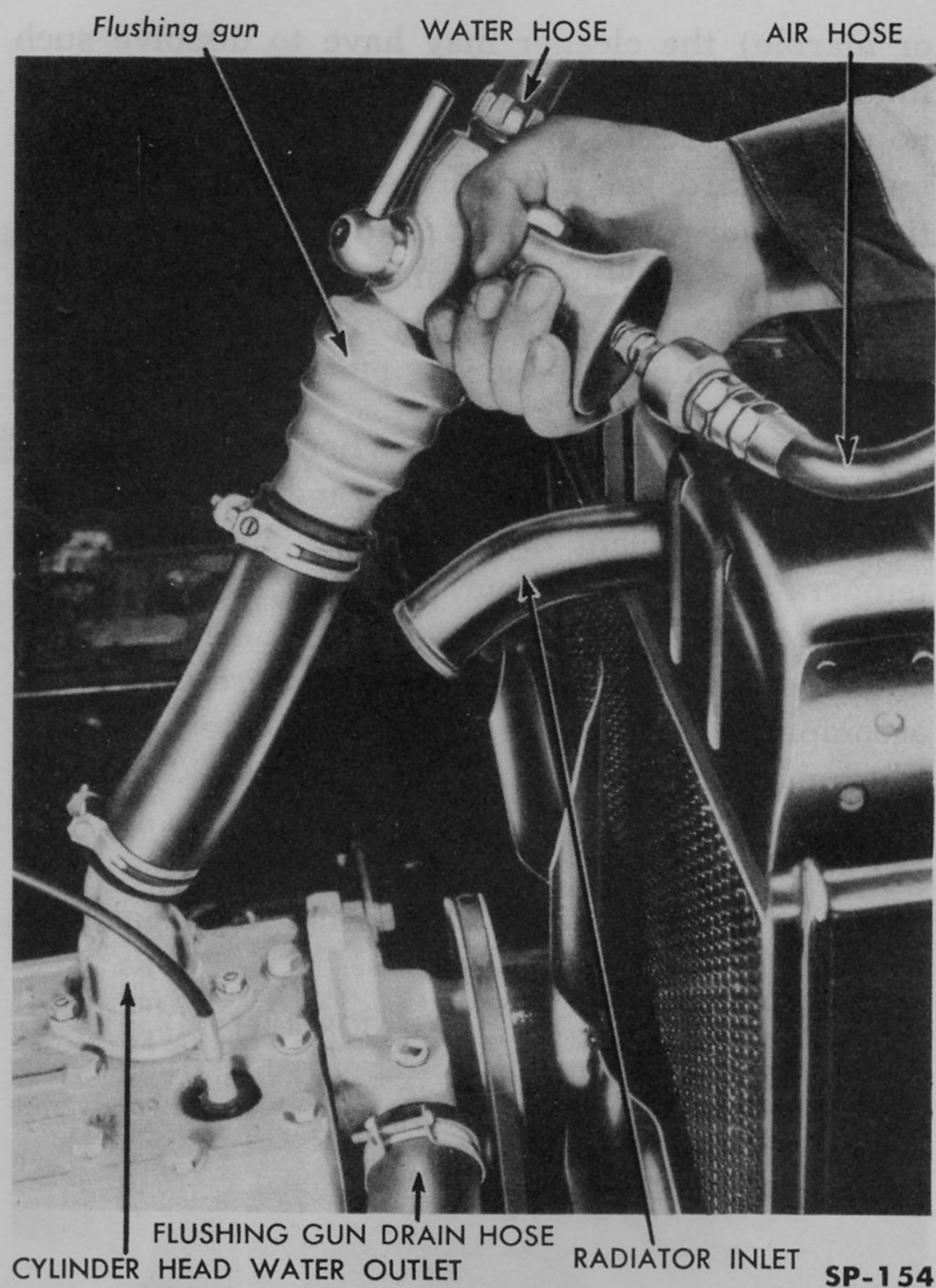
Fig. 163—Reverse Flushing Engine Water Jackets
