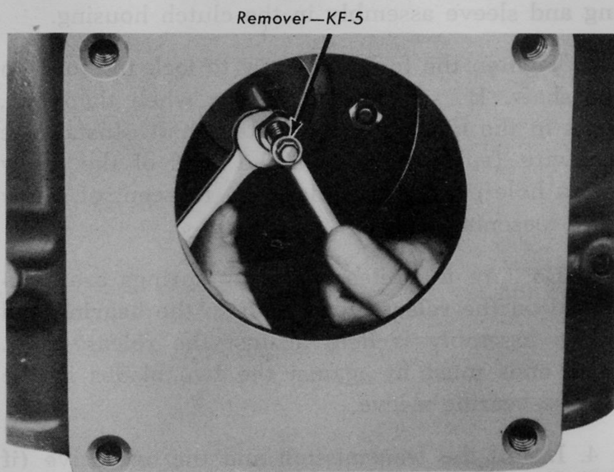
Fig. 176—Removing Crankshaft Pilot Bushing
