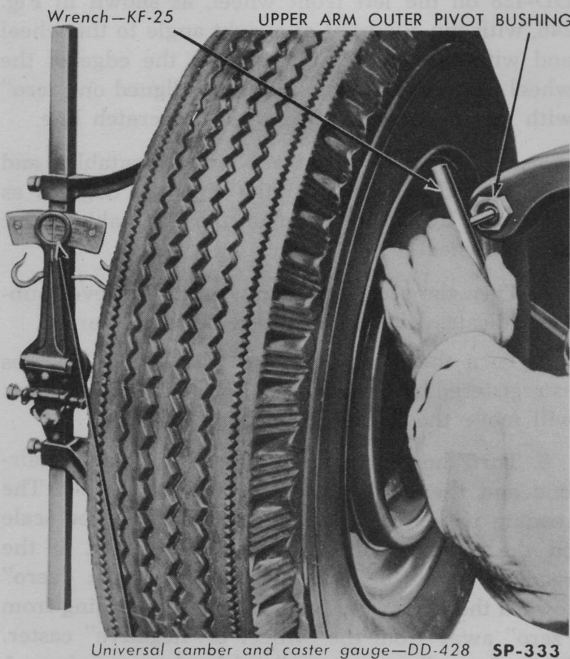
Fig. 247—Adjusting Caster or Camber at Upper Suspension Arm Outer Pivot
