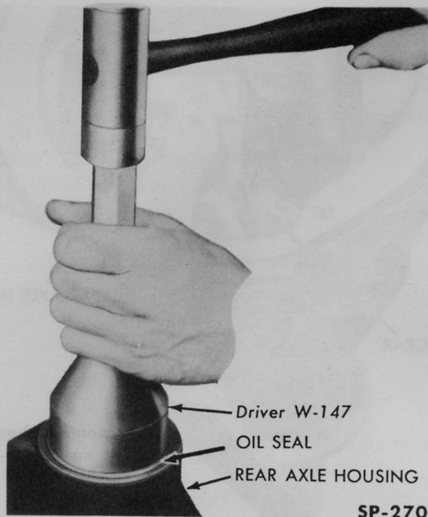
Fig. 274—Installing Pinion Oil Seal
