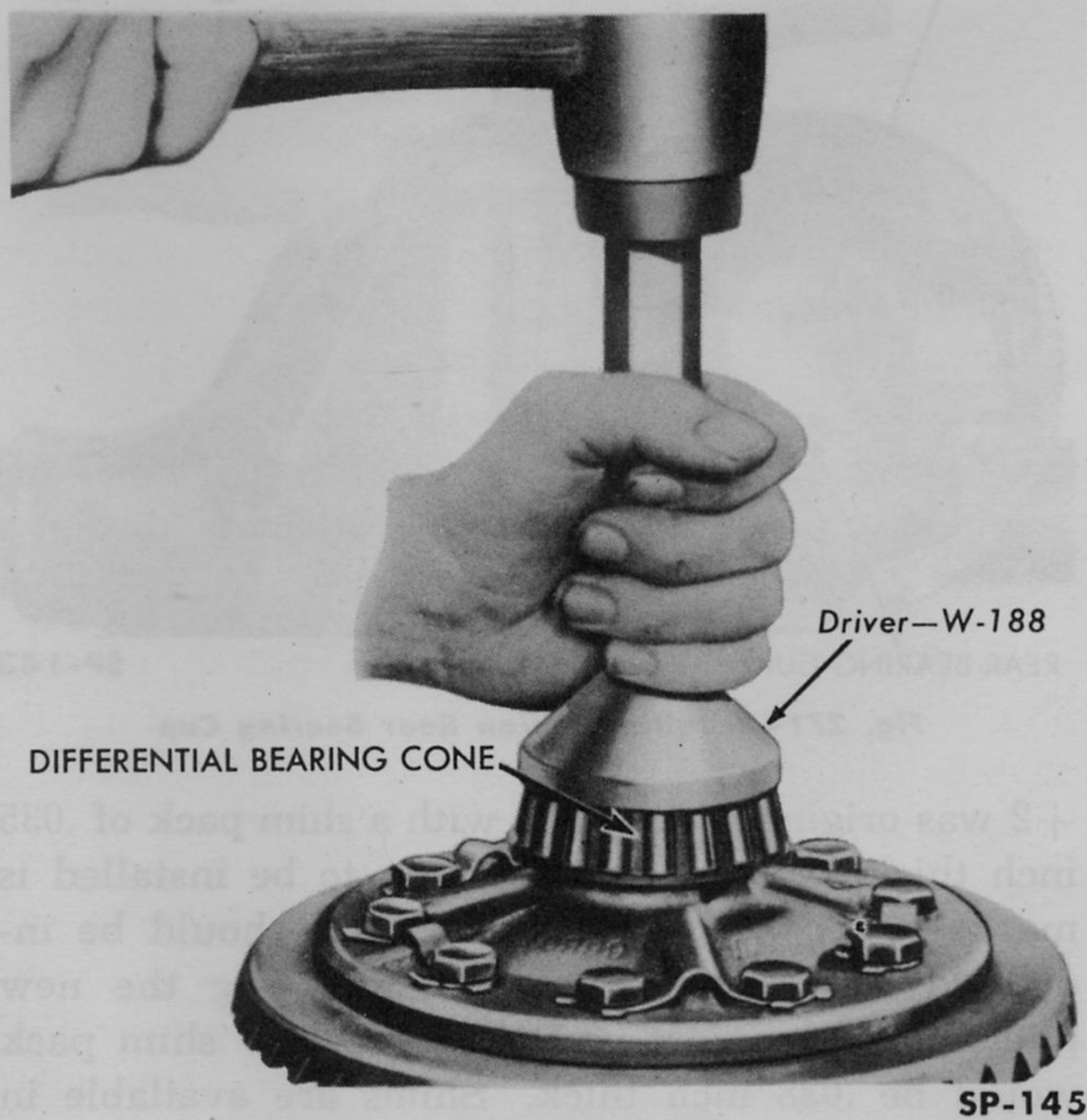
Fig. 267—Installing Differential Side Bearing Cone
