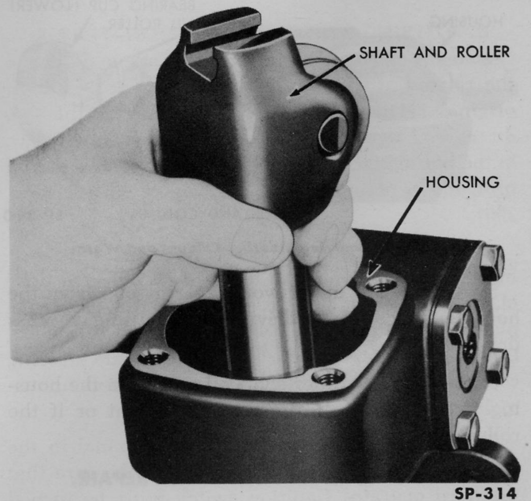
Fig. 292—Removing Shaft and Roller Assembly
