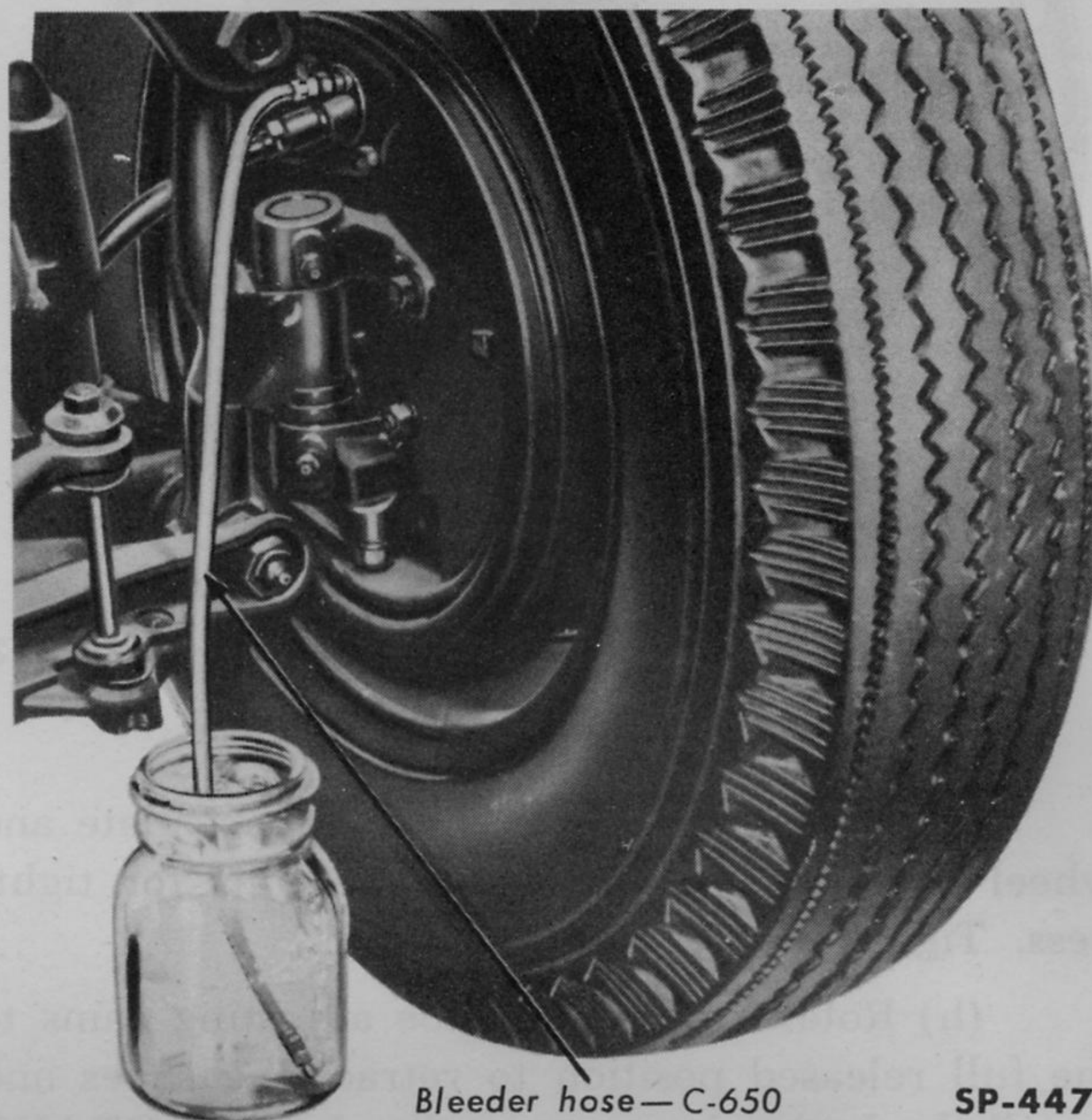
Fig. 303—Bleeding Hydraulic System at Wheel Cylinder
