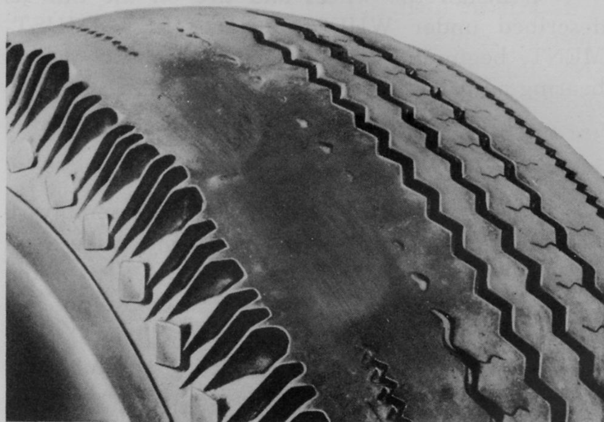
Fig. 317—Side or Camber Wear of Tire Tread
