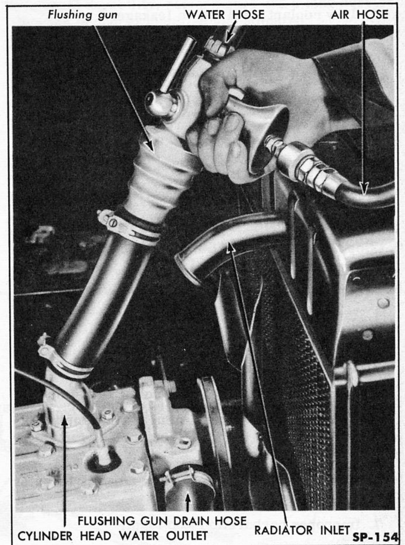
Fig. 102—Reverse Flushing Engine Water Jackets (Typical)
