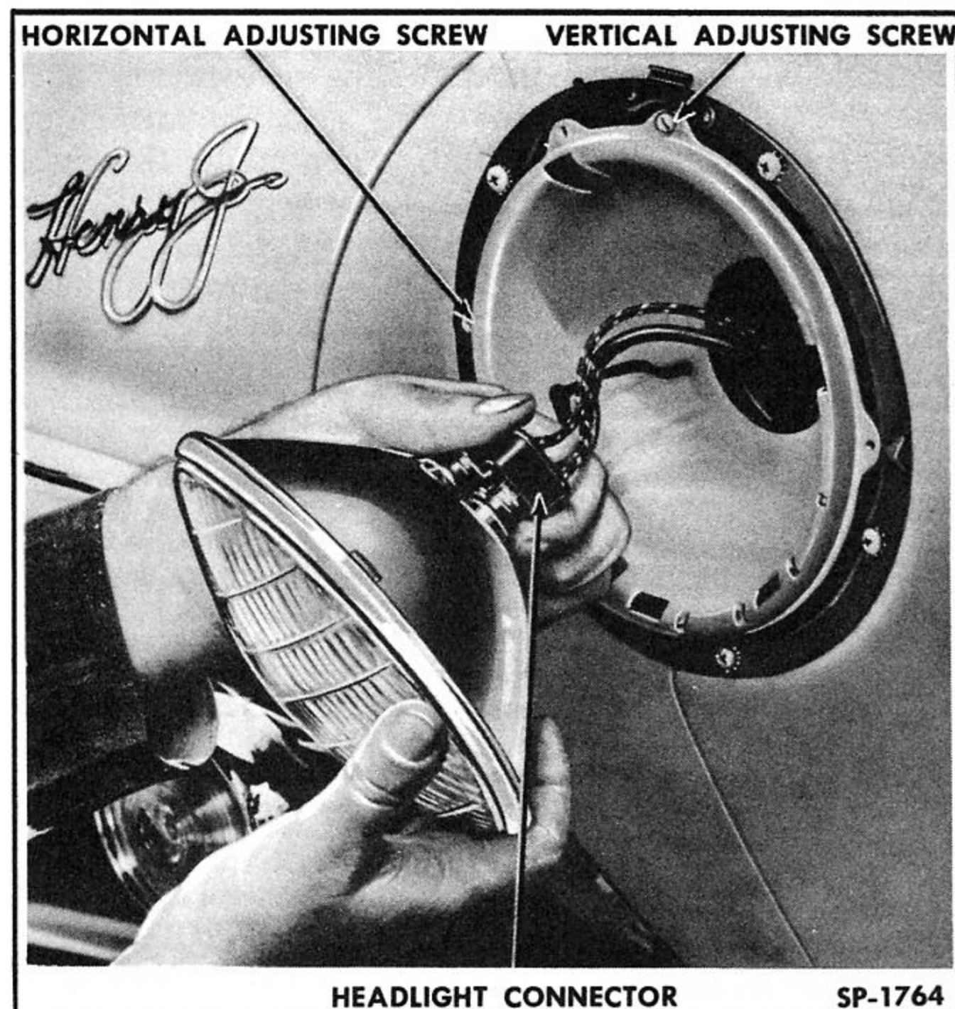
Fig. 305—Replacing Headlight Sealed-Beam Unit
