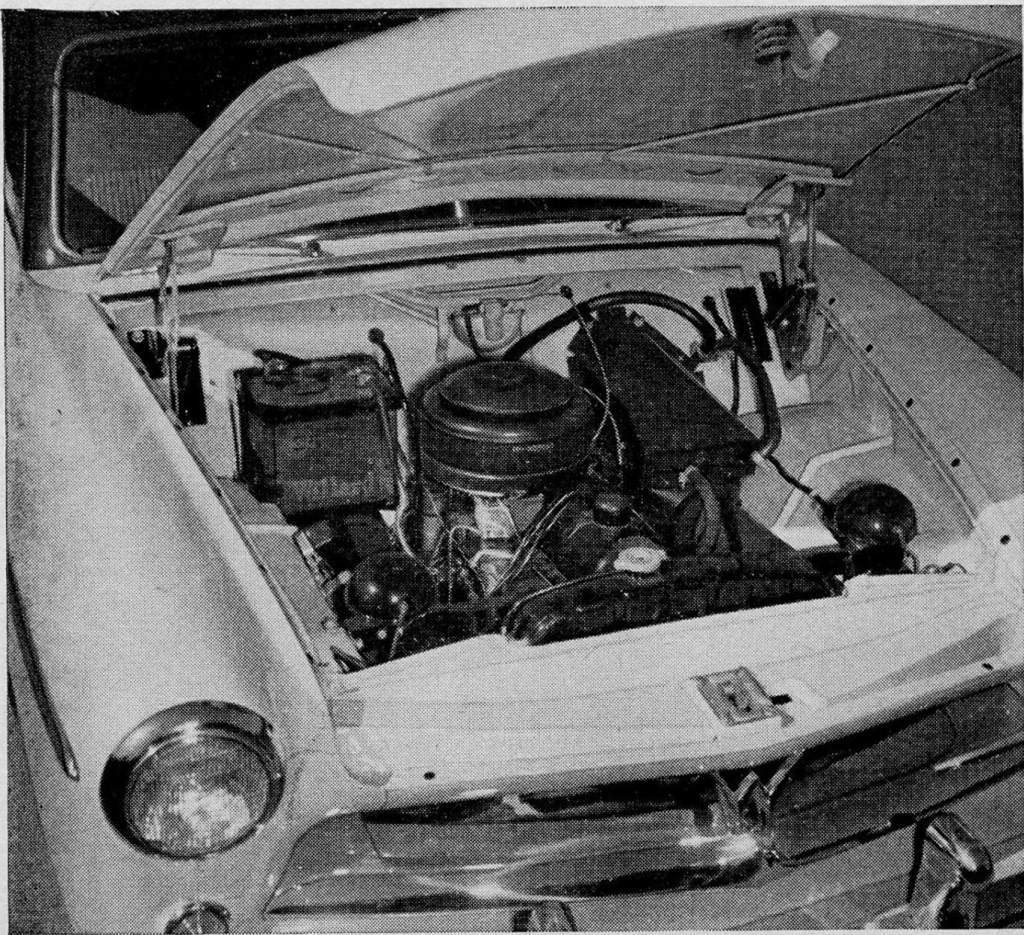
ENGINE has intake manifold cast integrally with block to eliminate gasket that might cause leakage. Cutaway (right) indicates position of single rocker arm for each cylinder, and extra-big intake valve.
