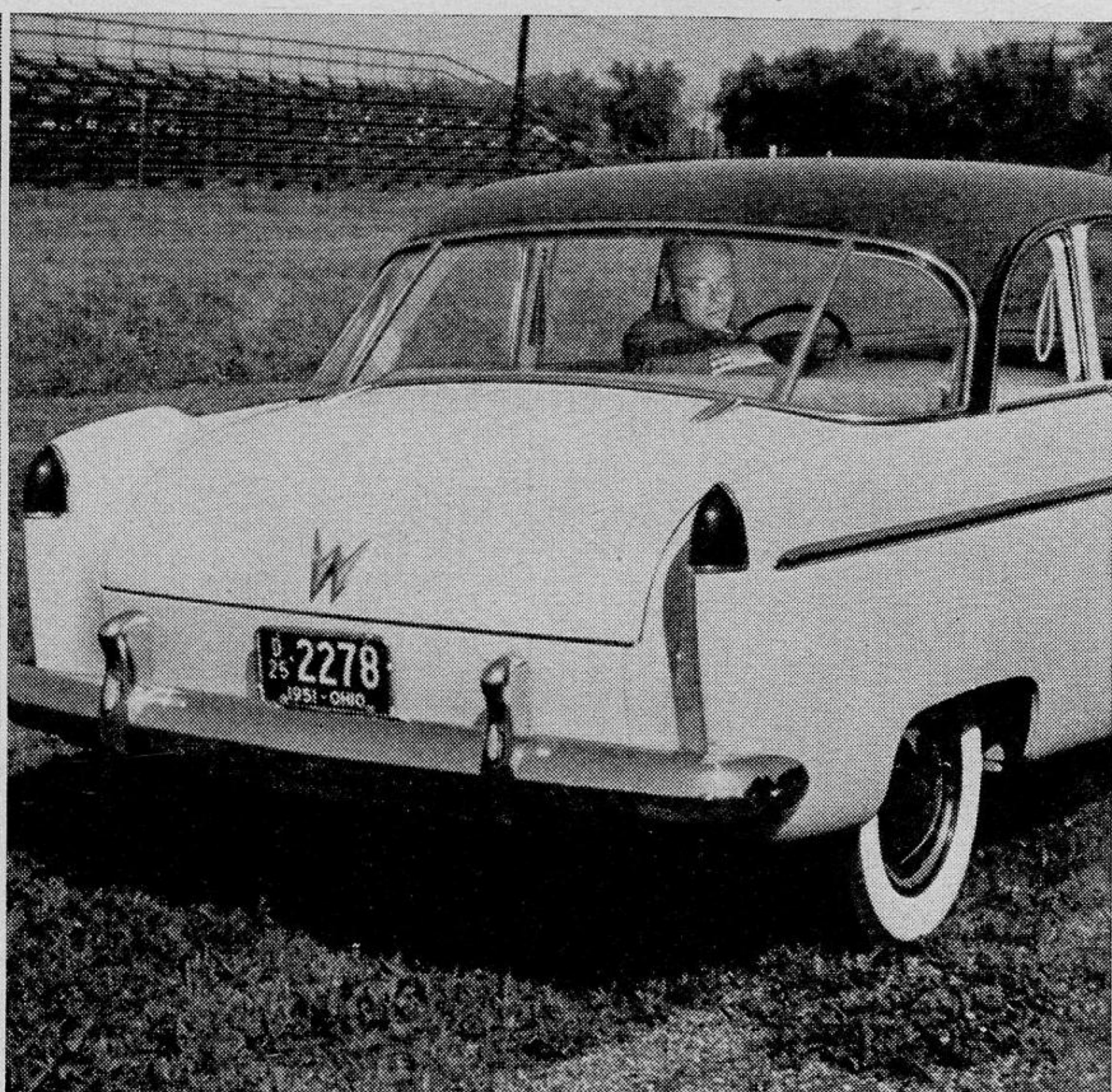
HERE'S A SURPRISE! Both rear fenders can be seen from driver's seat. On production models gas cap is next to license plate for easy access from either side.
