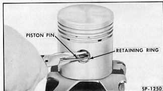
Fig. 11—Removing Piston Pin Retaining Rings
