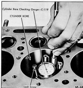
Fig. 9—Checking Cylinder Bore
