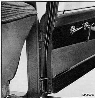
Fig. 41—Weatherseal Installation on Rear Door Hinge Pillar
