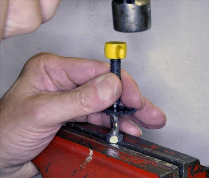
Swaging a gear plate
